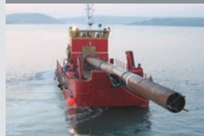
▲ 9 tonne steel pile in transit
